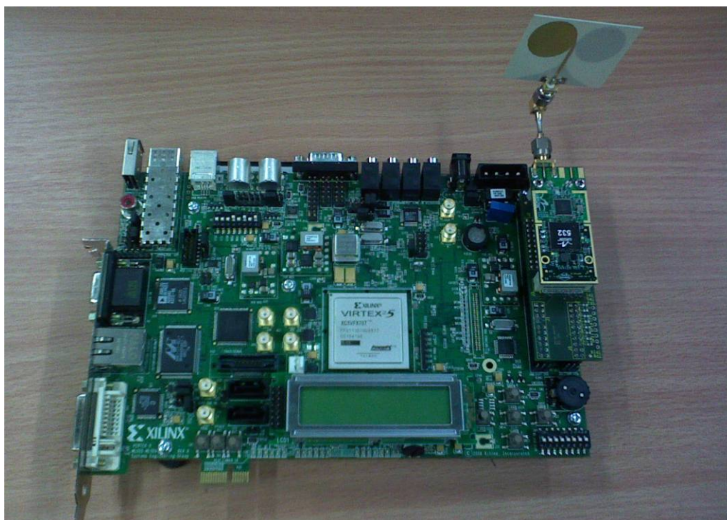
Figure 4-6: HDR “Open Platform” on a Xilinx ML507 Virtex-5
